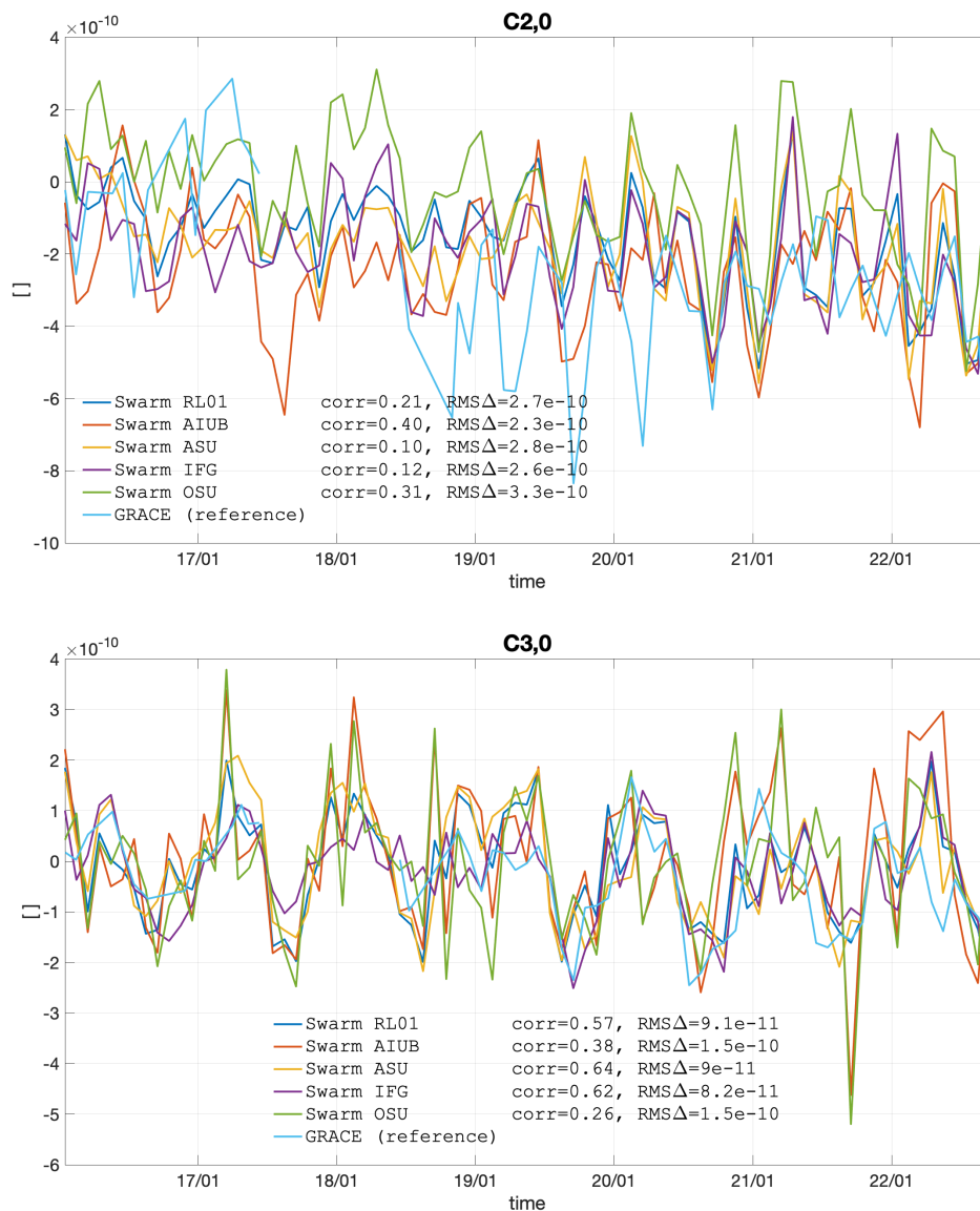
Figure 12 – Time series of the C_{20} (top) and C_{30} (bottom) coefficients, showing coefficients in the Swarm and GRACE/GRACE-FO GFMs. The statistics in the legend consider GRACE as reference.
